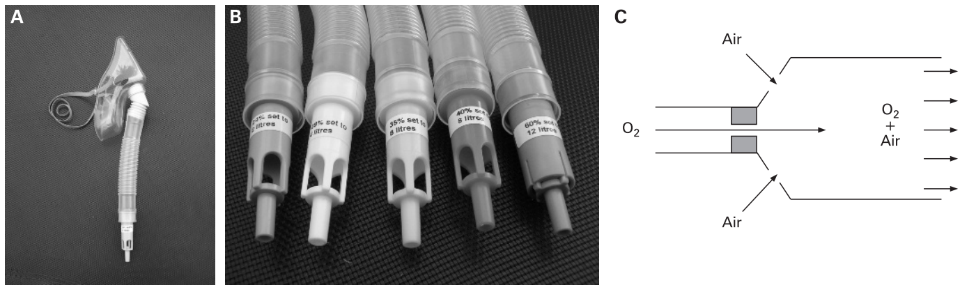
Figure 11 (A) Venturi mask. (B) Range of concentrations available. (C) Operation of Venturi valve. For 24% Venturi mask the typical oxygen flow of 2 l/min gives a total gas flow of 51 l/min. For 28% Venturi mask, 4 l/min oxygen flow gives a total gas flow of 44 l/min (table 11).
